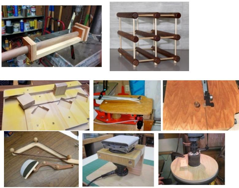
**Chris Voien** made this alignment jig so he could drill accurate holes for dowels when he made this wine rack. **Rubin Johnson** made a puzzle box known as the Impossible Dovetail Box. Rubin made a jig so he can accurately cut it with a router. It has to be accurate. Now he can make many of them.
