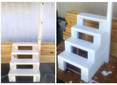
The Pictures are of a project that I was hired to do for one of my neighbors. They asked for a small set of stairs for assistance getting into and out of bed. The Stairs are made out of pine and are about 14 inches wide and 19.5 inches high. The handlebar is 44 inches high. Each stair has three ½ inch deep grooves for traction. Under each stair there is a finger groove to help with moving forward or back. The overall weight is also light enough to move.
